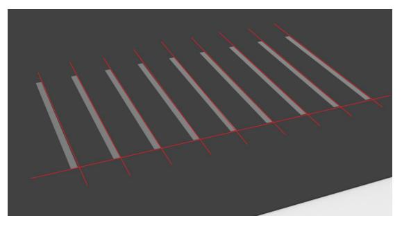
■ Paste the tube on the butyl tape and ensure full contact with it.
